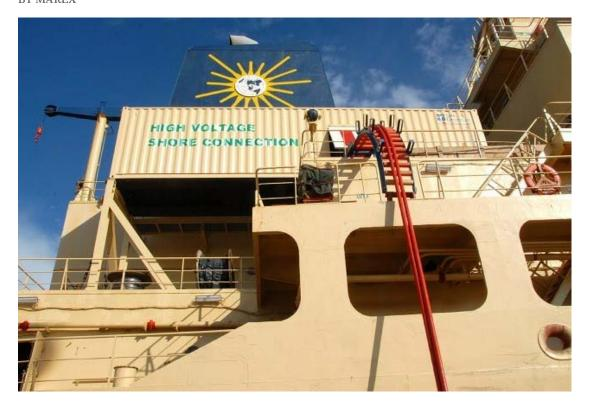
The Port of San Diego has successfully switched on its new shore-power system at the Tenth Avenue Marine Terminal, which will improve air quality and reduce greenhouse gas emissions by allowing cargo vessels to "plug in" rather than run their diesel engines while in port.
