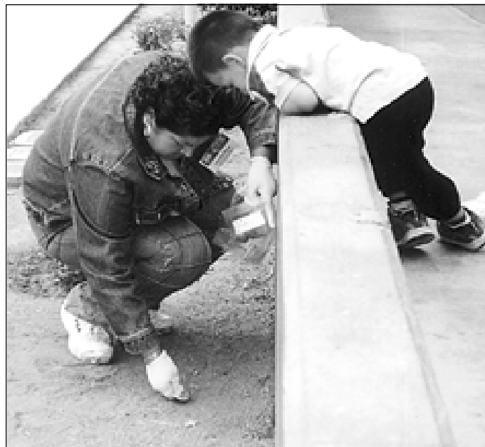
EHC Promotora Imelda Perez, left, conducts sampling to test for lead in soil surrounding one of EHC's project homes. EHC's Promotoras are certified lead sampling technicians and are also trained in the identification of other household hazards like mold, pests, and carbon monoxide.
